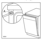
If your water is level 4 or 5, open the door and drill membrane (A) on the upper left-hand corner of the machine.
